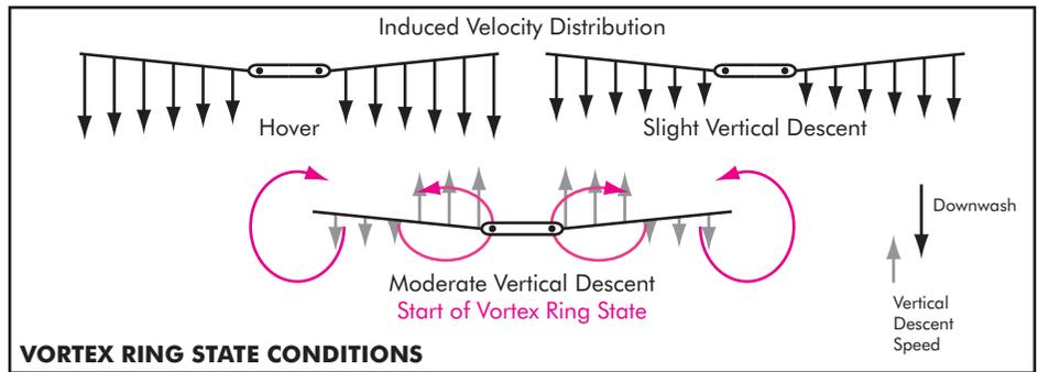
into the rotor system to blow the tip vortices away from the rotor and free it from the clutches of the vortex-ring state.
